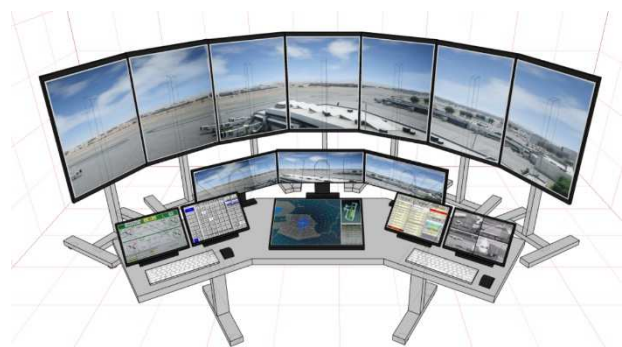
Fig. 9. Ergonomic 3D model of the Remote Tower simulator. Source: own
