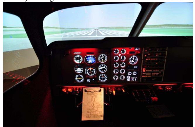
Fig. 4. Elite S612 BITD ME Simulator with flight model Beech Be58
